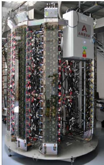
A 650W , 352.2 MHz module Developed by SOLEIL using 6 th Gen. LD MOSFET.
